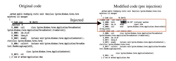
Note that this is a "pre injection" technique, in which our code is injected at the **beginning** of the original method code.
