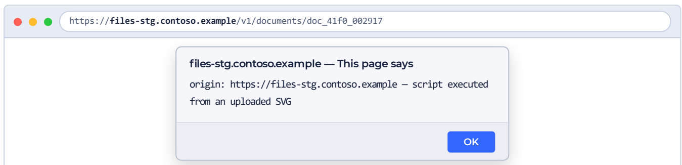
Figure 37. An uploaded SVG containing a script element is served inline and executes on the file service's own origin. ( Browser, staging )
